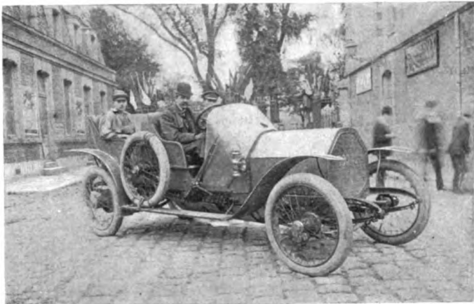
ARIES DRILLED THE FRAME AND FITTED A WIND DEFLECTOR.
